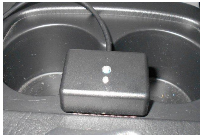
The neat IMA boost device in its case mounted with self adhesive Velcro near the cup holder.
