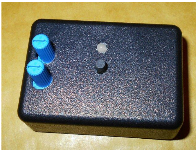
The IMA boost device in its case. Note the reverse mounted external access assist and regeneration level potentiometers in this example.
