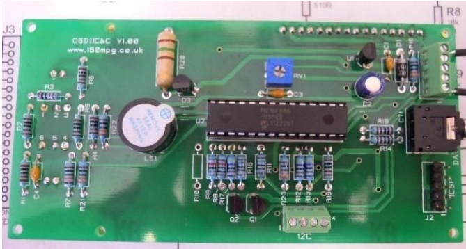
Rear view of the OBDIIC&C printed circuit board.
