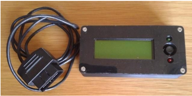
The hand-built Insight-specific OBDIIC&C unit in its bespoke 3D printed case.
